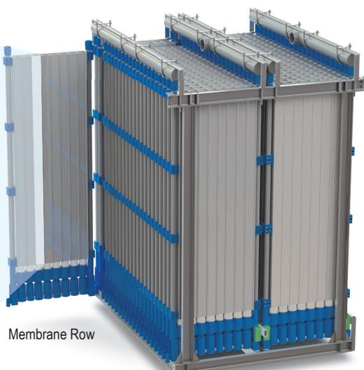
The simplified design of the PULSION MBR uses 40% less aeration energy to pulse a large bubble through a chambered fiber bundle creating a piston like pumping action that is more efficient and requires a smaller system footprint than previous models.
